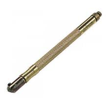
• Perfect cutting of glass - 2-valve technology - roung cutting head - cutting angle 158 degrees - straight edge stand-off distance 6mm - glass thickness up to 19mm
