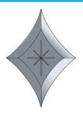
Regalead decorative glass bevels are designed primarily for the overlay market and are manufactured from 5mm float glass which is bevelled down to a 1.5  $\tilde{A}$  $\square$  1.8mm edge. These fine edges make the bevel pieces ideal for using with self adhesive lead but also suitable for customers working with traditional lead cames or copper foils.
