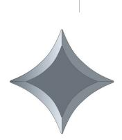
Regalead decorative glass bevels are designed primarily for the overlay market and are manufactured from 5mm float glass which is bevelled down to a 1.5  $\tilde{A}$  1.8mm edge. These fine edges make the bevel pieces ideal for using with self adhesive lead but also suitable for customers working with traditional lead cames or copper foils.
