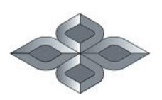
Regalead decorative glass bevels are designed primarily for the overlay market and are manufactured from 5mm float glass which is bevelled down to a 1.5  $\tilde{A}$  1.8mm edge. These fine edges make the bevel pieces ideal for using with self adhesive lead but also suitable for customers working with traditional lead cames or copper foils.
