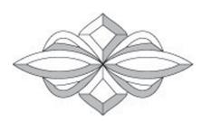
• Regalead decorative glass bevels are designed primarily for the overlay market and are manufactured from 5mm float glass which is bevelled down to a 1.5 - 1.8mm edge.
