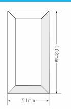
• Regalead decorative glass bevels are designed primarily for the overlay market and are manufactured from 5mm float glass which is bevelled down to a 1.5 - 1.8mm edge.
