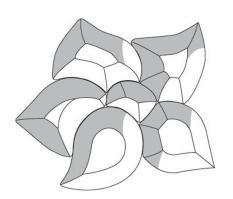
• Regalead decorative glass bevels are designed primarily for the overlay market and are manufactured from 5mm float glass which is bevelled down to a 1.5 - 1.8mm edge.
