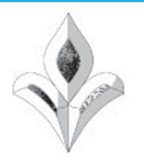
• Regalead decorative glass bevels are designed primarily for the overlay market and are manufactured from 5mm float glass which is bevelled down to a 1.5 - 1.8mm edge.
