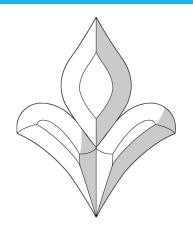
• Regalead decorative glass bevels are designed primarily for the overlay market and are manufactured from 5mm float glass which is bevelled down to a 1.5 - 1.8mm edge.
