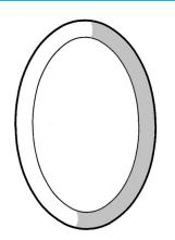
• Regalead decorative glass bevels are designed primarily for the overlay market and are manufactured from 5mm float glass which is bevelled down to a 1.5 - 1.8mm edge.
