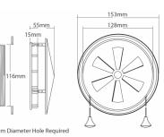
The Vent-A-Matic is a durable and effective in-glass ventilator that can solve most ventilation requirements. The 102 Rotary Vent is equipped with a diffusing rotor which helps to prevent severe drought and improve fresh air distribution within the room. The rotor also continues to operate whilst under its own inertia, even when air pressure on each side has been equalised.
