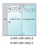
OP=Overpanel width SP=Sidepanel width DP=Door panel width
