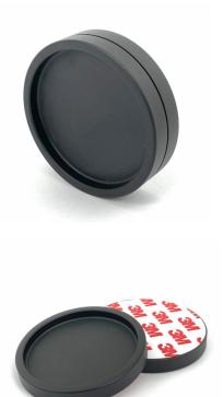
• 64mm diameter door pull can be easily mounted using the strong 3M tape with no need to drill the glass therefore reducing the cost of the glass processing.
