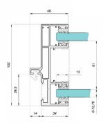
Suitable for glass thicknesses of 8-10mm.
