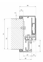
This stud/wall to glass door aluminium door frame with integrated hinge & receiver profile is suitable for glass thicknesses of 8-10mm.
