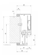
This stud/wall to glass door aluminium door frame with integrated hinge & receiver profile is suitable for glass thicknesses of 8-10mm.
