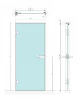
This Anodised L-type aluminium door frame with integrated hinge & receiver profile is suitable for glass thicknesses of 8-10mm.
