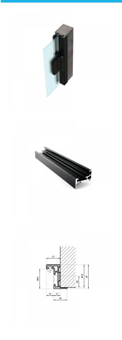
This Black Z-type aluminium door frame with integrated hinge & receiver profile is suitable for glass thicknesses of 8-10mm.
