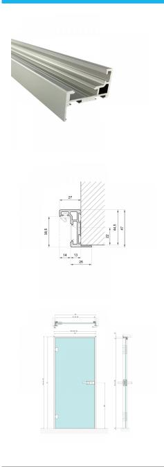
This Anodised Z-type aluminium door frame with integrated hinge & receiver profile is suitable for glass thicknesses of 8-10mm.
