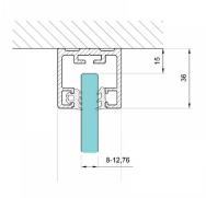
Aluminium glass partition system for use on the top.
