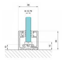
Aluminium glass partition system for use on the bottom and side.
