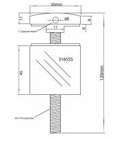
• Stainless steel point fixture suitable for mounting glass panels both vertically and horizontally.
