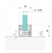
Aluminium glass partition system for use on the bottom and side.
