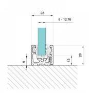
Aluminium glass partition system for use on the bottom and side.
