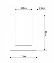
U channel suitable for 10mm thick glass.
