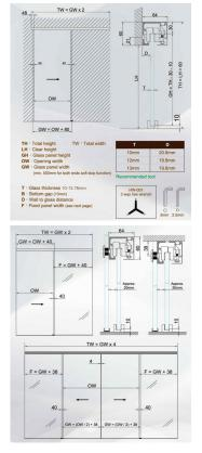
• An ultra slim profile suitable for wall, ceiling or glass mounting.
