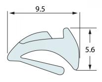
• Tear Off Clear Dry Glazing Wedge Gasket - Thin - Clear
