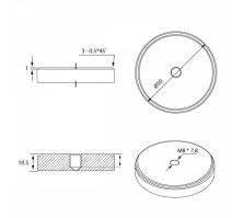
• 50mm Dia Stainless Steel Discs 50mmx10.5 M8
