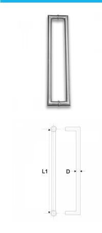
• Dimensions Hole Centers - 600mm 12-16mm holes required Diameter - 32mm
