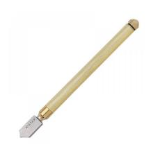
1. Unsurpassed in quality, this High precision tools offer the greatest value in Hand held cutters avaliable anywhere 2. Tungsten Carbide wheel, perfectly ground to 138 degree and exactly fitted on a Tungsten Carbide axle to provide cleanest score and longest Wobble free service life 3. Unique oil feed system controls oil amount to suit the individual user's requirements
